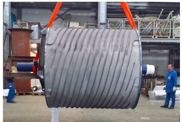
Fig.2: Coating of casting rollers (up to \varnothing 3.200 \text{ mm} )
