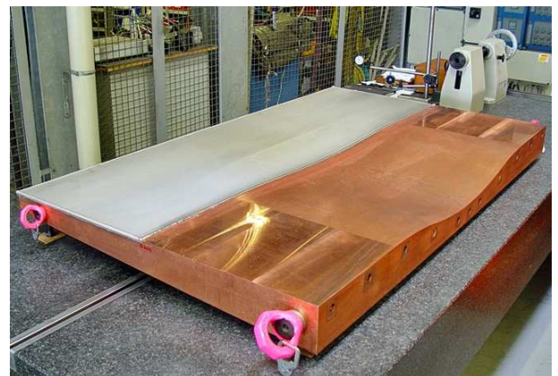
Fig.5: Ingot Mould with 5000 \mu\text{m} Nickel Sulfamate
