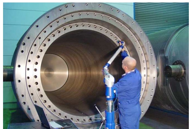
Fig.3: Inside coating of CASTOR containers (96 t)
